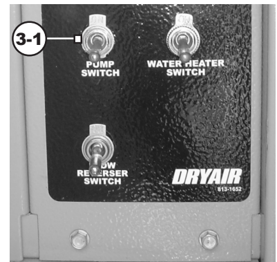
3 - pump, water heater & flow reverser switch
