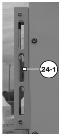
24 - glycol level gauge
