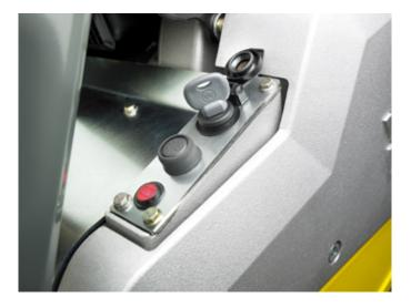
Available with crank handle or electric starter. The electric starter model is conveniently started with an ignition key.
