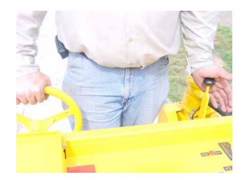
Drive the drill unit to the edge of the slab where the two wheels along the edge are parallel to the edge, and the edge of the slab is just under the black round Tool Bar.
