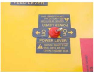
Turn the first drill on by placing the individual power switch into the "On" position. The corresponding drill will start drilling. The drill should move forward into the concrete with a slight "quiver" as it drills. If it is "bouncing", it means it does not have enough feed pressure. Lift up and slowly turn the regulator knob clockwise until the "bouncing" stops and you still have good rotation on the bit.
