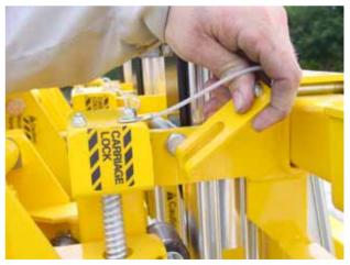
Place the "Raise and Lower" valve into the "lower" position.
