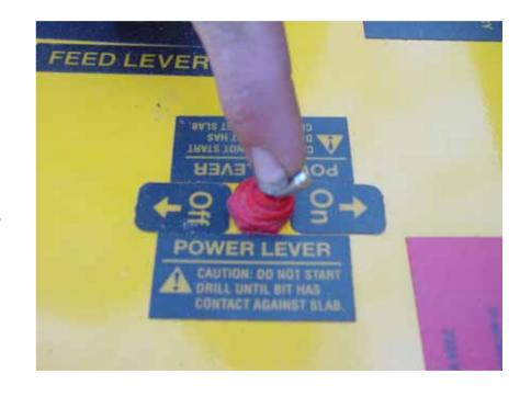
After each drill reaches its preset drill depth, it will shut off automatically. When all drills have shut off, place the Main Power Switch to the "Off" position.
