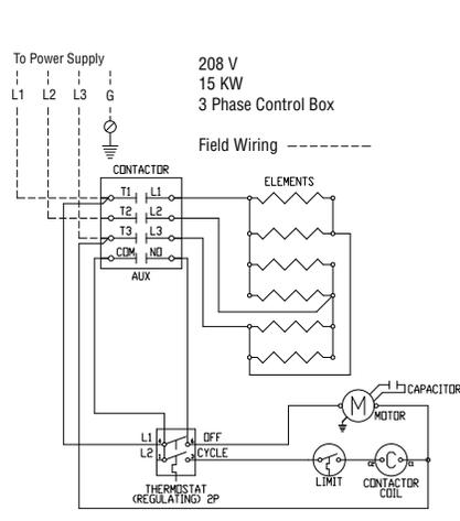
**Wiring Diagram 5 - 208V / 15KW, 3 Phase**
