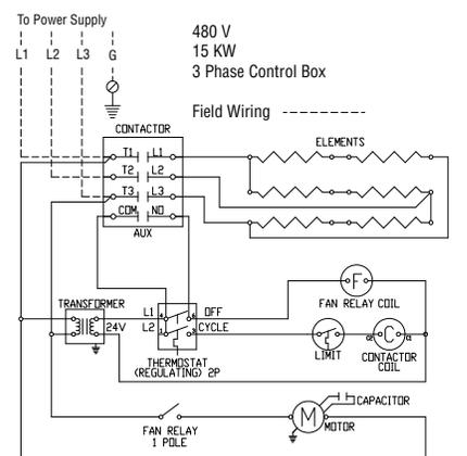
**Wiring Diagram 3 - 480V / 15KW, 3 Phase**
