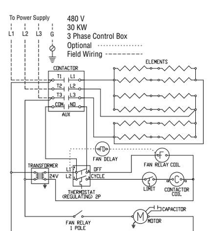
**Wiring Diagram 6 - 480V / 30KW, 3 Phase**
