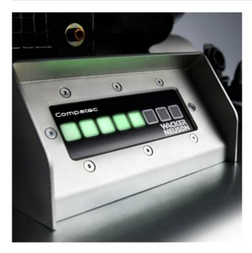
Compatec - Compaction Control **Available as an accessory**: Easy to read Compatec helps the operator determine when maximum compaction has been reached. The number of lights will increase with each pass and no longer increase once maximum compaction is achieved.
