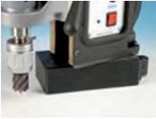
In order to permit optimum alignment even in difficult positions, the model MAB 845 is additionally equipped with a rotating mechanism. It allows the upper part of the machine to be rotated by 30° to both sides and by 20 mm forwards and backwards with the magnetic foot engaged.
