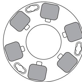
By changing the way the diamonds are set-up on the diamond holder discs, an operator can significantly effect the performance of the machine and therefore, the finished product.
