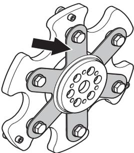
Replacement spring steel springs are available and can be replaced without throwing the grinding head away.
