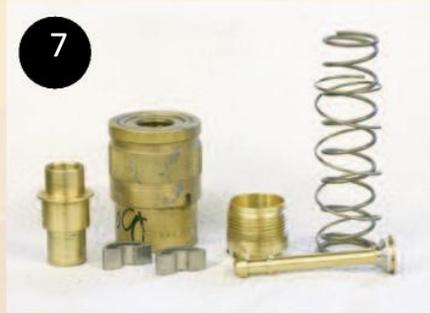
Pictured above are all parts from the disassembled coupler
