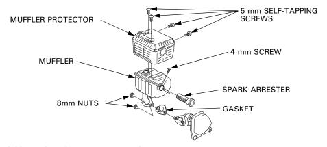
4.Use a brush to remove carbon deposits from the spark arrester screen. Be careful to avoid damaging the screen.
