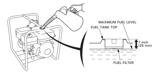
Refuel in a well-ventilated area before starting the engine. If the engine has been running, allow it to cool. Refuel carefully to avoid spilling fuel. Do not fill the fuel tank completely. Fill tank to approximately 1 inch (25 mm) below the top of the fuel tank to allow for fuel expansion. If may be necessary to lower the fuel level depending on operating conditions.
