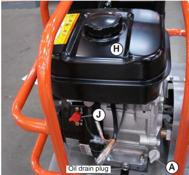
The oil drain plug is located at the bottom of the engine block. Place a pan under the drain and remove the plug. Drain the oil and replace the plug. Using a long neck funnel, fill the engine with 0.6 quarts (0.6 liters) of oil. When full, the oil level should be at the high level mark on the dipstick (A) or to the top of the threads on the engine fill hole. The engine is equipped with an oil alert system that will stop the engine if the oil level is low.
