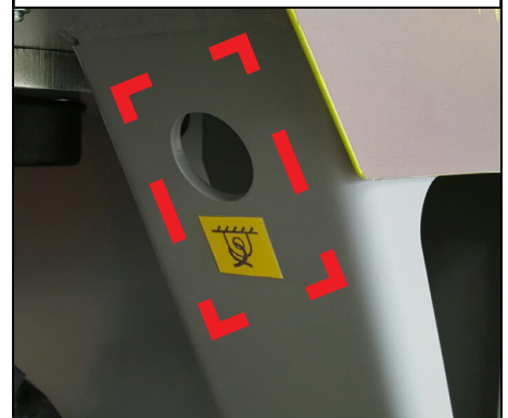
Fig 26: Anchor points located each side of the ED
