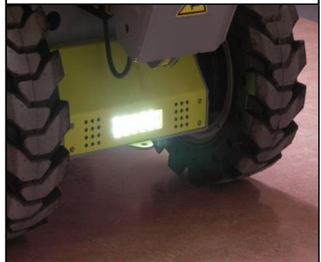
Fig 17: Ensure front facing lights are functioning and free from debris.
