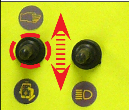
Fig 15: Remote Control .Up=ON /Down = OFF
