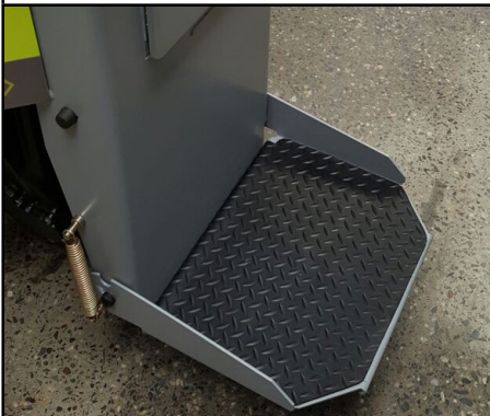
Fig 1: The ED platform in the DOWN position. When down, stand on the platform to operate the electric dumper
