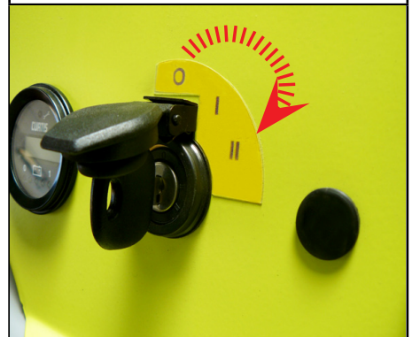
Fig 3: Turn the key clockwise to position II to start the ED.
