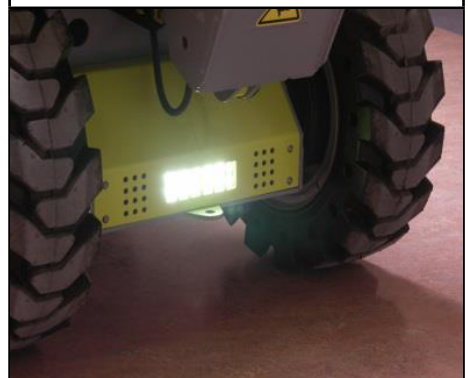
Fig 20: Ensure front facing lights are functioning and free from debris.
