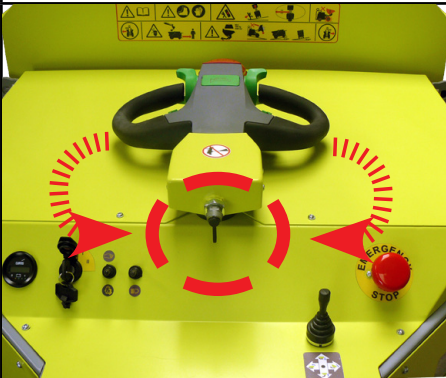
Fig 6: Speed Switch. Two options Creeper and Full.
