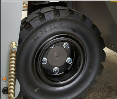
Fig 2: Tighten wheel nuts if loose to correct torque settings
