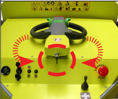
Fig 9: Speed Switch. Two options Creeper and Full.
