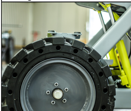
Fig 5: Tighten wheel nuts if loose to correct torque settings
