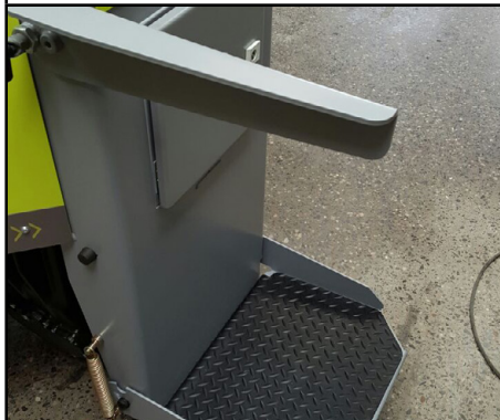
Fig 2: The ED with the safety rails up and locked into position.
