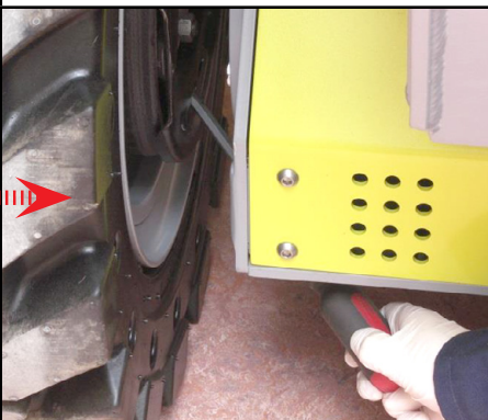
Fig 31: Adjust brake shoe as needed.
