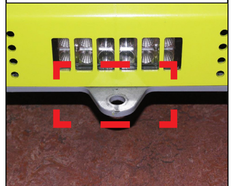
Fig 26: Anchor points located each side of the ED
