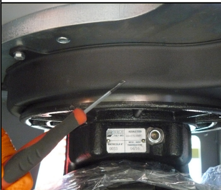
Fig 29: Remove side cover to grease rear drive unit gears.
