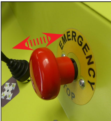
Fig 11: Emergency Stop Button("E-stop")
