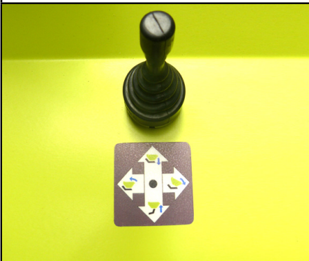
Fig 18: Remote Control. Up=ON /Down = OFF
