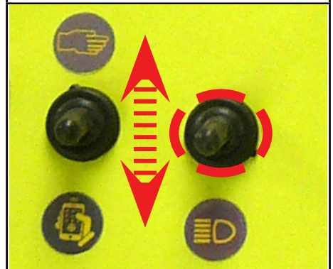
Fig 20: Ensure front facing lights are functioning and free from debris.
