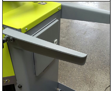
Fig 17: The ED with the safety rails up and locked into position.
