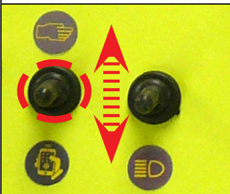
Fig 18: Remote Control. Up=ON /Down = OFF
