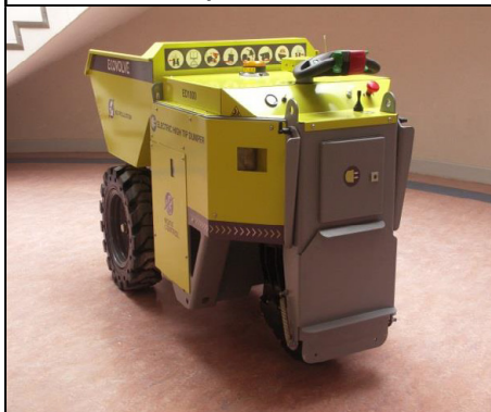
Fig 16: The ED platform in the up position. When UP , the operator can walk behind the electric dumper.
