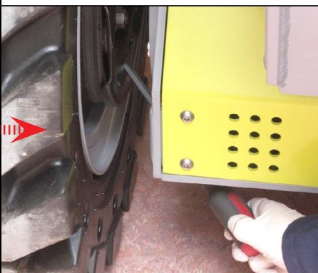
Fig 34: Adjust brake shoe as needed.
